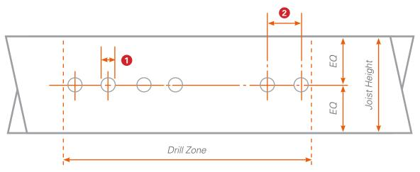
1 Maximum dia. of hole = Joist height x 0.25 2 Minimum distance between hole centres = Largest hole dia. x 3
