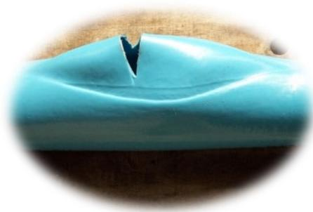
**Ductile rupture**, independent of time, a very high internal pressure can exceed the strength of the pipe causing it to stretch and fail in a ductile way.
