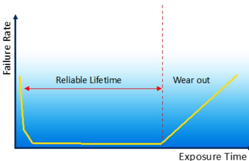
UK experience shows that drinking water pipes will exhibit the late life failure modes sooner than gas pipes, as chlorine initiates an oxidation degradation mechanism. Research by water companies and manufacturers show that for the earlier generation materials transition to 'wear out' will likely start at around 235 years<sup>2</sup>.
