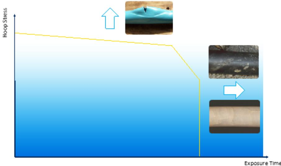
An envelope of performance can be constructed, using Arrhenius<sup>1</sup> equations, describing when these failure modes can occur in time.
