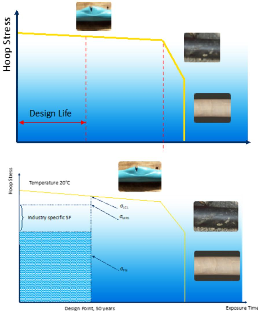
Design point: In the UK, in common with much of the world, the given time (the design point) is 50 years. The strength is predicted from test data at an operating temperature 20°C.
