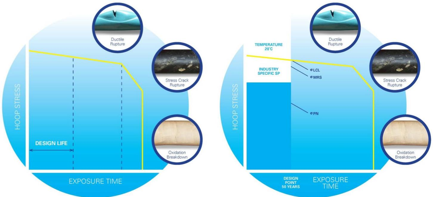
In the experience of the UK, it is likely drinking water pipes will exhibit the late life failure modes soonest. This is because chlorine ultimately initiates an oxidation degradation mechanism. Research by water utilities and manufacturers shows that for earlier generation materials the transition to wear-out mode will likely start at around 235 years.<sup>2</sup> For other applications like natural gas or hydrogen, oxidation onset should take considerably longer.
