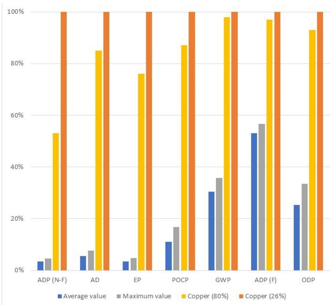
The greatest difference in the values between copper and plastic pipe is caused by the impact of production. So although recycling of copper (from off-cuts from site and at end of life) would save on extraction of raw materials, the environmental impact would still be much higher than any of the four plastic piping systems.
