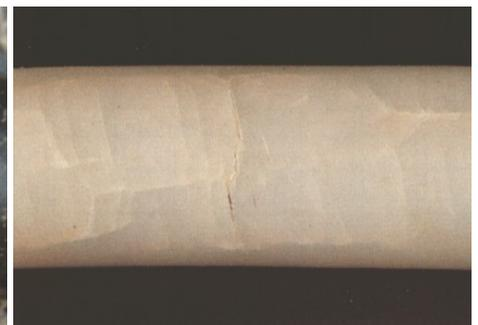
**Oxidation**, largely independent of pressure, at very long timescales, the likely reliable lifetime limit will be as a result of polymer oxidation.
