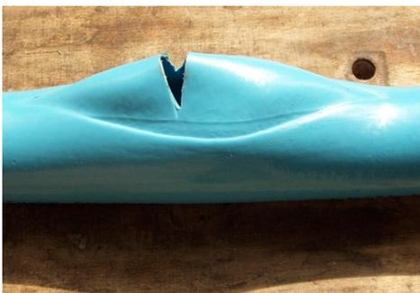
**Ductile rupture**, independent of time, a very high internal pressure can exceed the strength of the pipe causing it to stretch and fail in a ductile way.
