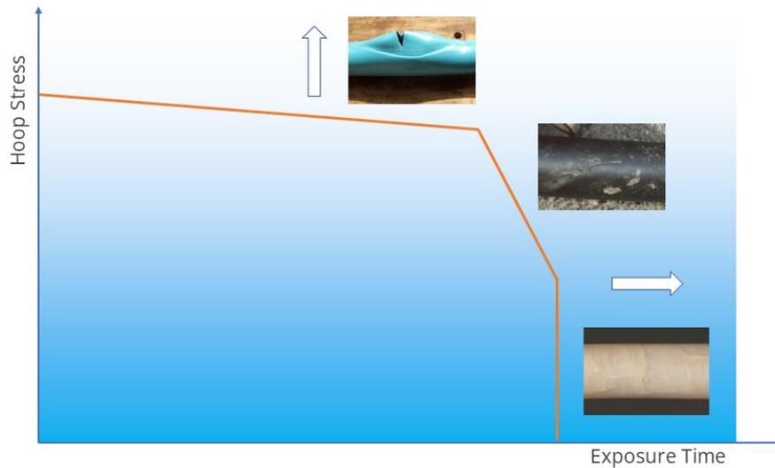
An envelope of performance can be constructed, using Arrhenius<sup>1</sup> equations, describing when these failure modes can occur in time.
