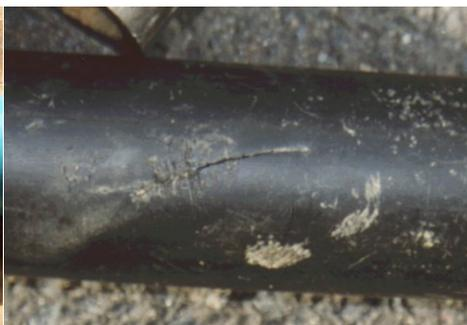
**Stress crack**, at lower pressures but much longer timescales, the reliable lifetime limit could be brittle crack grown through the material.
