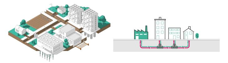
District heating is the concept of having one or more central heat sources instead of individual boilers. The heat is transported from the central heat source through a network of underground pre-insulated pipes to each building. Each building typically uses a heat interface unit (HIU) which will provide space heating and hot water to the building from the district heating network. The heat used is then metered to each building and consumers are billed for their energy use.
